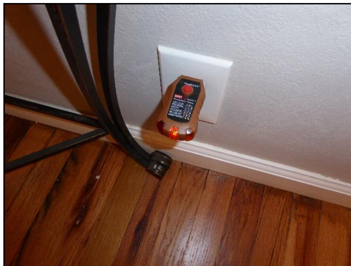
38. Ground needed for 3-slot outlet
