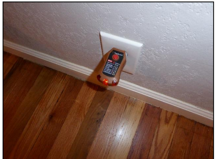
35. Ground needed for 3-slot outlet
